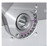
4. Place the adjustment key on the eccentric disc (hole circle) and turn it in the desired direction by one hole position.
